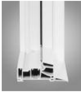
1-1/4" PVC jamb extension installed in the exterior accessory groove gives an overall (OAT) depth of 4-1/2" but sets the window back into opening by 1-1/4". Combine the two for a 5-3/4" overall (OAT) depth.
