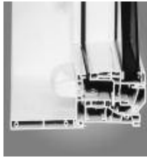
3-5/16" PVC jamb extension installed in the interior accessory groove gives an overall (OAT) depth of 6-9/16".
