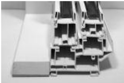
The addition of a composite jamb extension to the interior of the window allows the depth to be expanded from 4-1/2" to 9-3/4".
